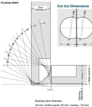
In case of door thickness up to 20 mm. Material: Particle board.
